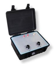
Burden for Current Transformer is mainly used for loading a CT during testing. Available in several structural designs for use in a variety of testing environments, this Burden for Current Transformer is compliant with IEC 60044-1 or ANSI/IEEE C57.13. Customer specifications can also be requested to satisfy different requirements.
