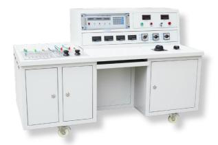
WHES Series Instrument Transformer Testing System is designed to measure various properties of electromagnetic current transformers and potential transformers (voltage transformers). The choice of actual components for the system can be custom-configured according to the types of tests and measurements needed, which can include ratio-error tests, phase-error tests, CT volt-ampere characteristic tests, PT (VT) no-load-loss tests, DC resistance tests, open-circuit voltage tests, etc.
