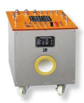
WHLB Series Standard Current Transformers are mainly used as reference CTs for current transformer measurements and tests: error tests, characteristic tests, and so on. These reference current transformers, available in various accuracy levels, are in compliance with IEC 60044 (IEC 61869) or ANSI/IEEE C57.13. They can also be made according to other requirements and specifications.
