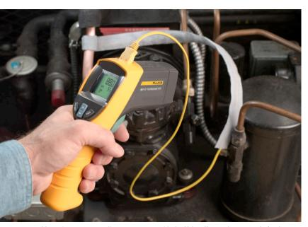
Measuring compressor line temperature with the Velcro K-type thermocouple for the Fluke 561 IR Thermometer.
