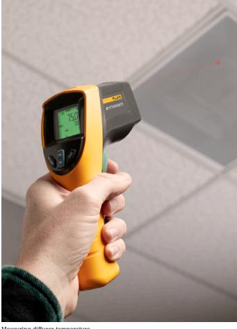
Measuring diffuser temperature.
