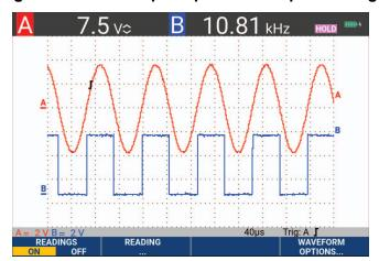
Figure 6. Hz and V peak-peak as Scope Readings
