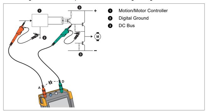
Figure 40. Parasitic Capacitance Between Analog and Digital Reference
