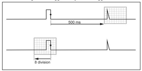
Figure 26. Trigger Delay or Pre-Trigger View
