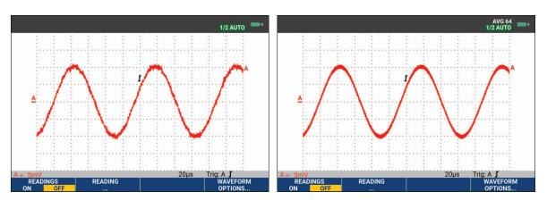
Figure 7. Smoothing a Waveform
