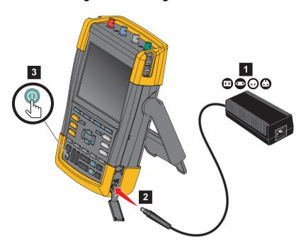
Figure 1. Powering the Test Tool
