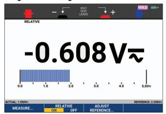
Figure 16. Making a Relative Measurement
