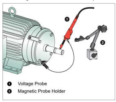
Figure 35. Motor Shaft Test Setup
