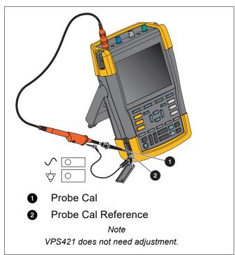
Figure 48. Voltage Probe Adjustment
