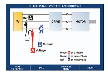
Figure 34. MDA-550 Connection Diagram
