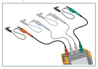
**Figure 4. Scope Connections**
