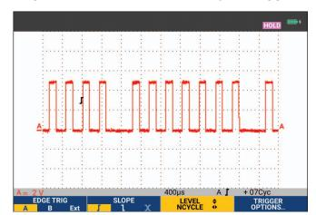
Figure 28. Waveforms with N-Cycle Trigger
