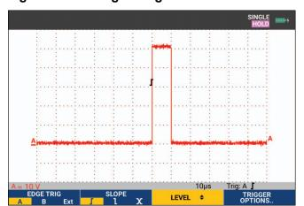
Figure 27. Making a Single Shot Measurement
