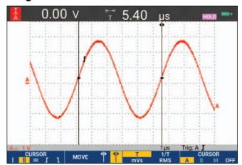
Figure 23. Time Measurement with Cursors
