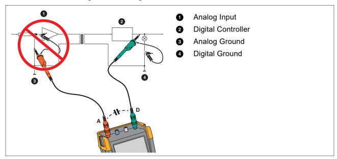
Figure 42. Wrong Connection of Reference Leads
