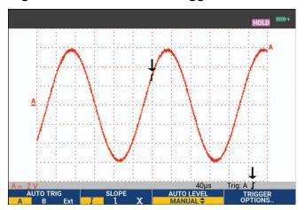
Figure 25. Screen with all Trigger Information
