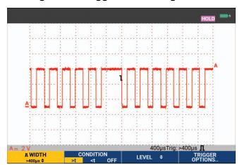
Figure 30. Trigger on Missing Pulses
