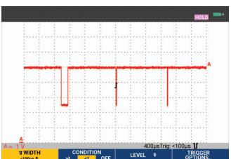
Figure 29. Trigger on Narrow Glitches
