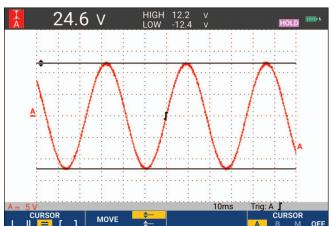
Figure 22. Voltage Measurement with Cursors
